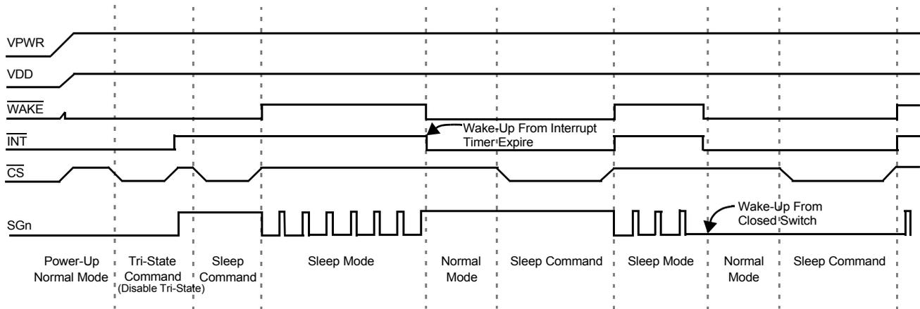
Figure 5. Sleep Mode to Normal Mode Operation
