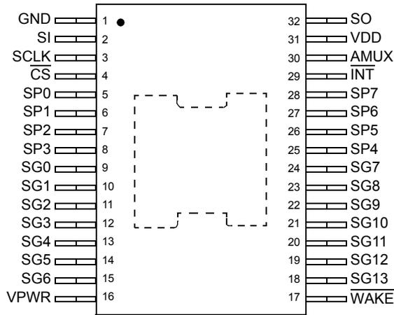
Figure 3. 33975 Pin Connections
