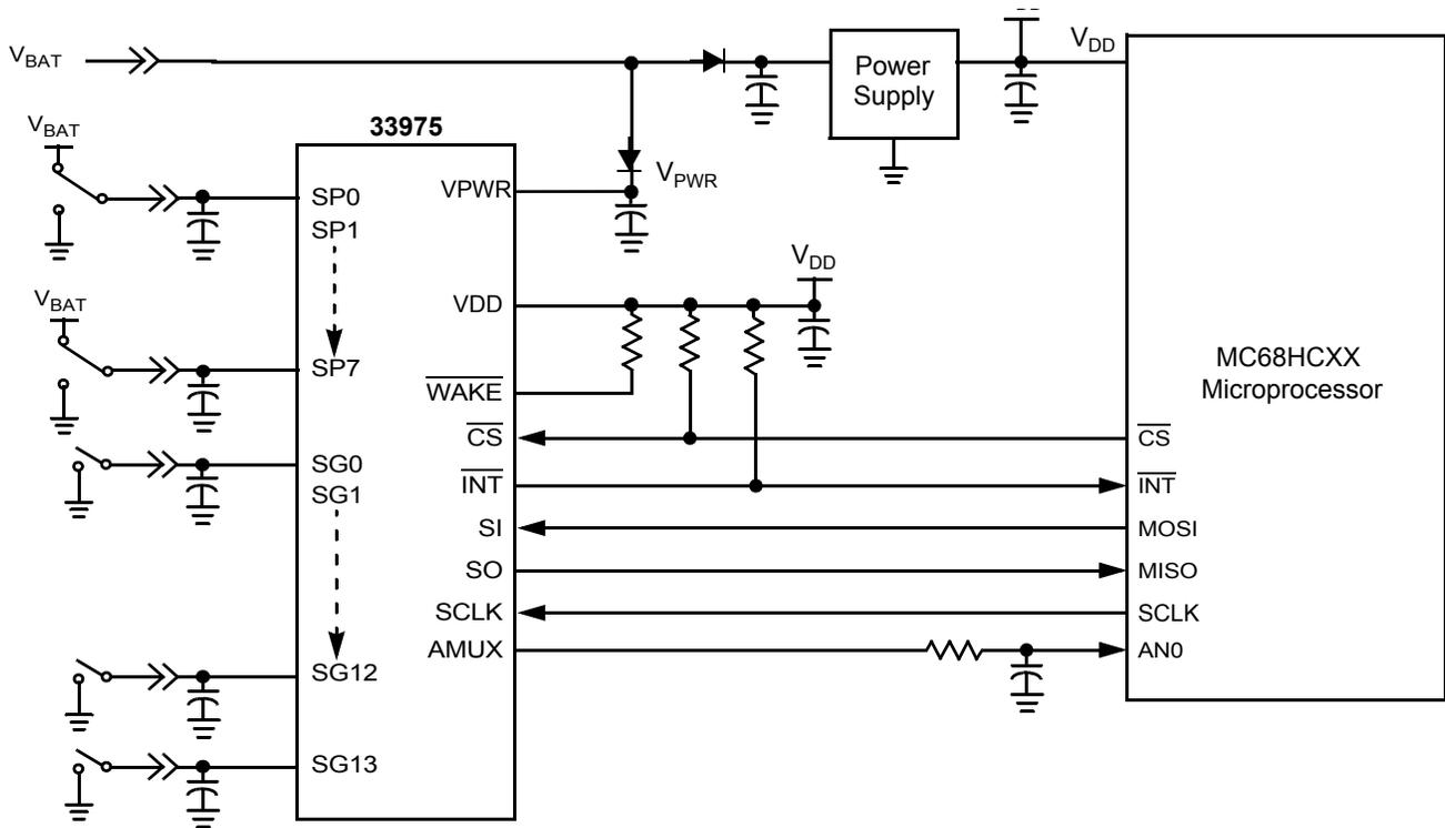
Figure 16. Power Supply Active in Sleep Mode
