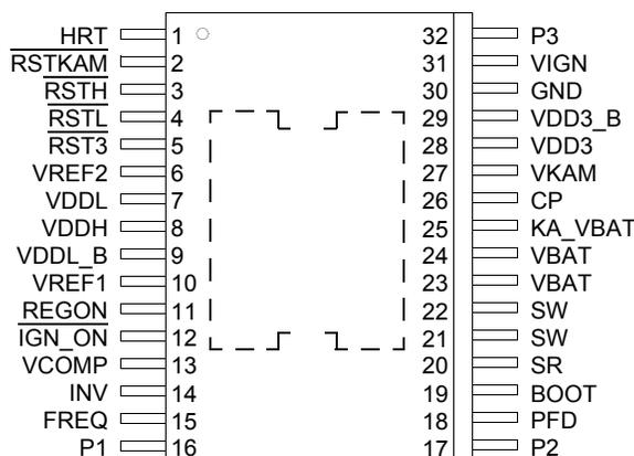
Note: The exposed pad is electrically and thermally connected to the IC ground.
