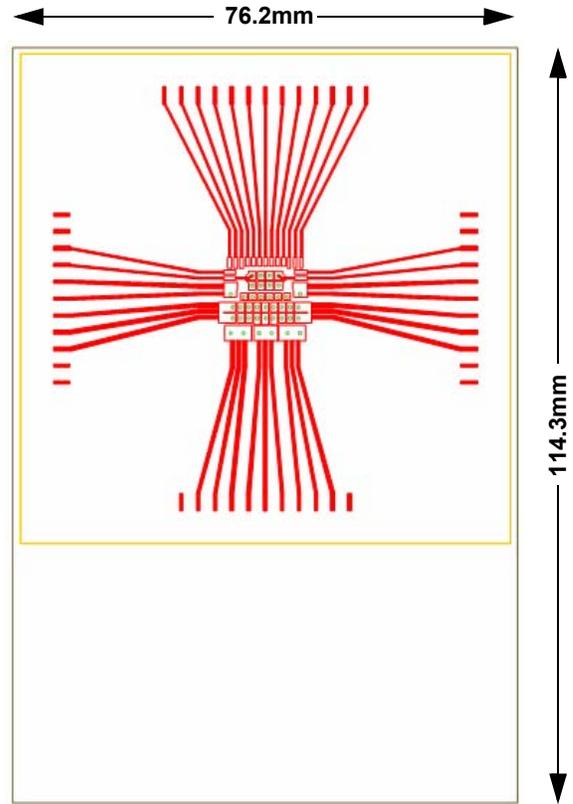
Figure 18. 2s2p JEDEC Thermal Test Board
