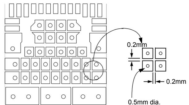
**Figure 16. Detail of Copper Traces Under Device with Thermal Vias**
