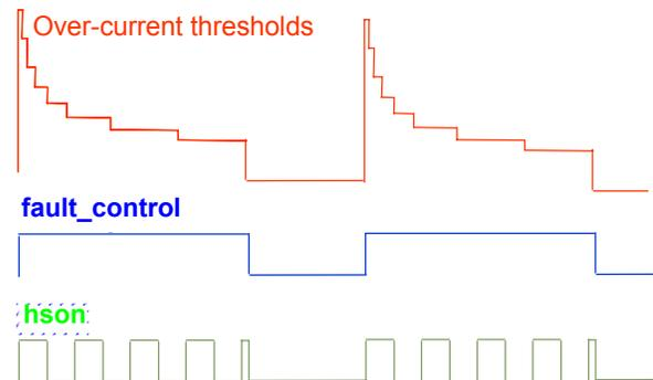
In steady state, the wire harness will be protected by OCLO2 current level by default. Three other DC over-current levels are available: OCLO1 or OCLO3 or OCLO4 based on the state of the OCLO[1,0] bits.
