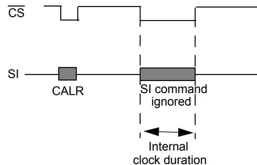
In case of negative  $\overline{CS}$  pulse is outside a predefined time range (from  $t_{CSB(MIN)}$  to  $t_{CSB(MAX)}$ ), the calibration event will be ignored and the internal clock will be unaltered or reset to default value ( $f_{PWM(0)}$ ) if this was not calibrated before.
