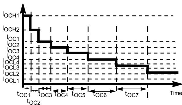
**Figure 14. Over-current Profile Depending on Xenon Bit**
