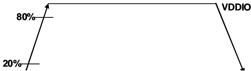
Figure 4. Output Pad Transition Waveform
